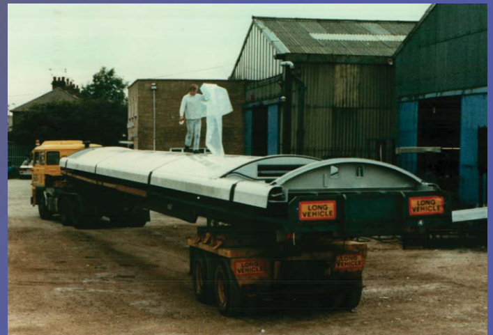
Roof assembly ready for delivery.
